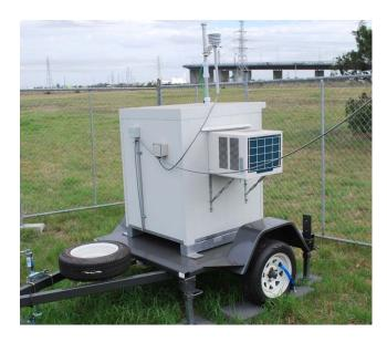
Dust monitoring - During construction, onsite monitors measure dust and local conditions to assist in managing the contractor's works and dust suppression program.
